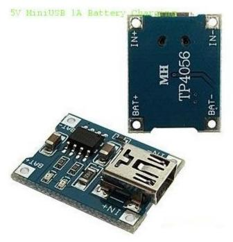
Description: 100% band new and high quality Charge module- Linear charging Current- 1A adjustable Charge precision- 1.5% Input voltage- 4.5V-5.5V Full charge voltage- 4.2V Led indicator- red is charging blue is full charged Input interface- mini USB Work temperature- -10°C to +85°C Inversed polarity- NO Size- small to 25X19X10mm NOTE:
